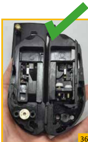
To adjust the width of the lock on side B, press the lock.
