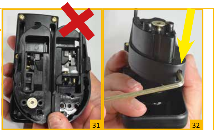
Left side(B) is yet not adjusted in keeping with the right(A). Case height adjustment screw.
