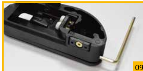
Activate the lock lever, putting it in lock mode.
